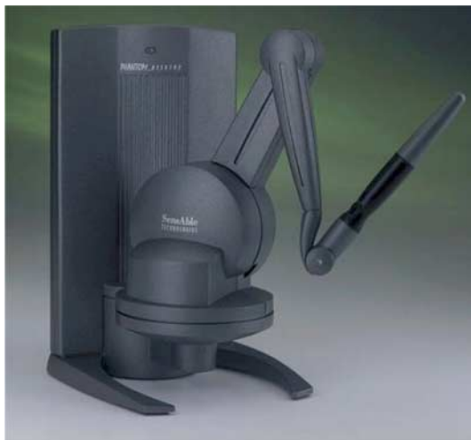
Figure 2. PHANTOM ® desktop device from SensAble Technologies, Inc (Woburn, MA, USA).
